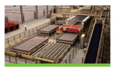
Among the six production lines, five are standard production lines that can produce WWCB of varying thickness from 10 to 100mm. The other large wall component production line principally manufactures 3m x 6m x 40cm large wall components which can be installed directly. It is the most advanced and fully automated production line in the world.
